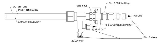
Figure 4-1. Catalytic Cartridge
